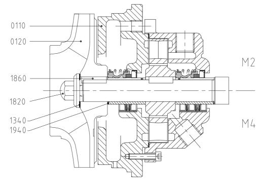
Figuur 23: Disassembling the impeller.
