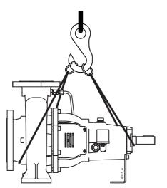
*Figure 2: Lifting instructions for single pump.*
