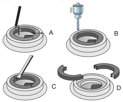
Figure 24: Removal of wear ring.
