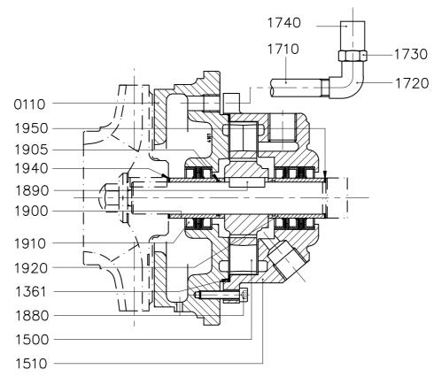
Figure 35: Parts of shaft sealing group M4.
