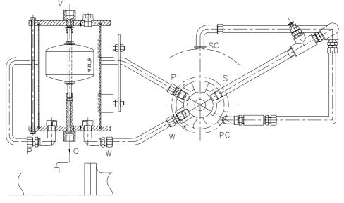
Figure 32: Dimensions pump with float de-aerator.
