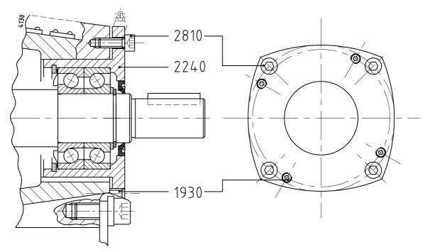
Figure 28: Adjustment of the axial play.
