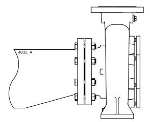
Figure 6: Eccentric reducer to suction flange.
