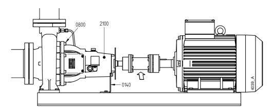
Figure 17: Back-Pull-Out principle.
