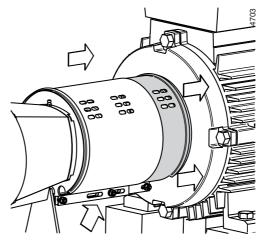
*Figure 22:* Adjusting the jacket at motor side.
