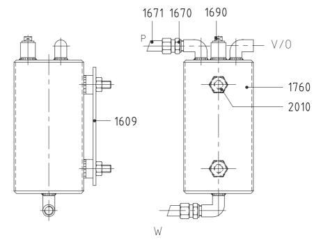
Figure 36: Parts of service liquid tank TL.
