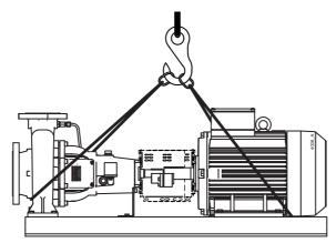
Figure 1: Lifting instructions for pump unit.
