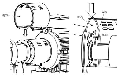
Figure 21: Fitting the jacket at pump side.
