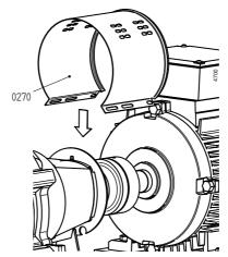
Figure 18: Fitting the jacket at motor side.
