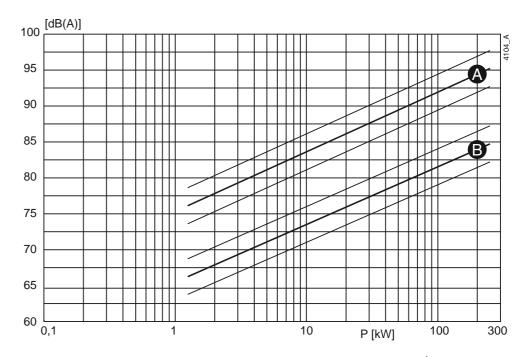
Figure 44: Noise level as function of pump power [kW] at 2900 min<sup>-1</sup> A = sound power level, B = sound pressure level.
