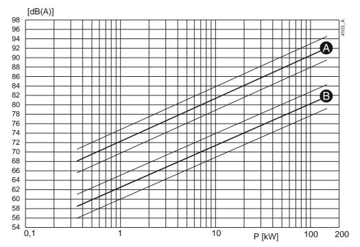
*Figure 43:* Noise level as function of pump power [kW] at 1450 min<sup>-1</sup> A = sound power level, B = sound pressure level.
