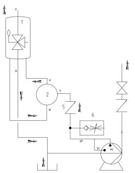
Figure 12: Connection diagram with float-controlled de-aerator.
