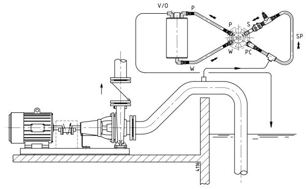
*Figure 10:* Medium: thin, clean and slightly polluted liquids. In case part of the suction pipe lies higher than the pump, venting should also be provided in this part. If the suction pipe is short, or the lift in the suction pipe small, venting at the highest point is not necessary. However, the suction time will be longer.
