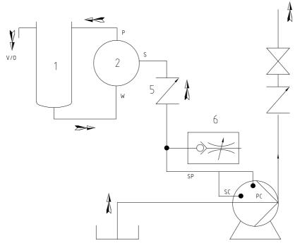
Figure 7: Connection diagram with service liquid tank.
