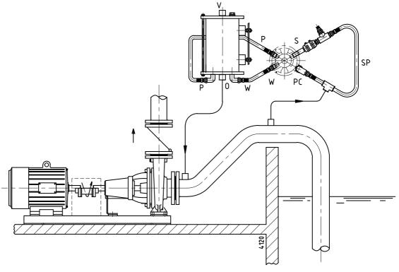
*Figure 15:* Medium: thin, clean and slightly polluted liquids. In case part of the suction pipe lies higher than the pump, venting should also be provided in this part. If the suction pipe is short, or the lift in the suction pipe small, venting at the highest point is not necessary. However, the suction time will be longer.
