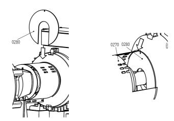
*Figure 19: Fitting the assembly plate at motor side.*
