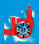
Petroland pumps use a rotor with sliding vanes that draw the liquid in behind each vane, through the inlet port and into the pumping chamber.
