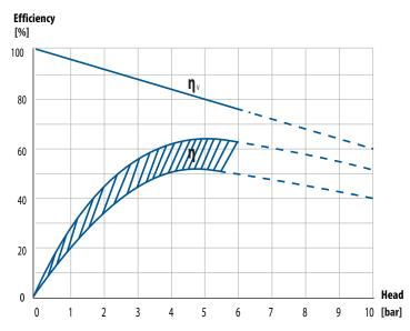
Volumetric efficiency nv and overall efficiency n on pompe 3P Hollow Rotory Disk pumps
