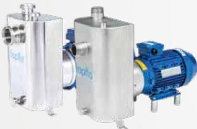
The CTS series maintains all the benefits and strengths of the standard CT pump. The self-priming feature allows to use the pump in applications where standard CT pumps do not prove useful. The CTS pump is capable of creating up to 4,5 m of suction lift. By replacing only one element – the casing with a self-priming chamber – we can achieve various advantages for our pump. The pump can now suck the liquid from a lower level than it is positioned or handle liquids with high content of air.
