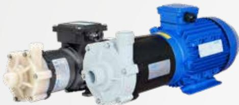
CTM is a compact and seal less pump, where the power from the motor is transmitted to the impeller by means of a magnetic coupling. The wetted components are non-metallic injection moulded thermoplastics PP-GF or PVDF. The pumps handle many types of low viscous clean liquids such as chemical aggressive and toxic ones.
