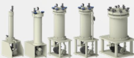
Cartridge filters with 1, 3, 7 or 15 cartridges are stand alone units equipped with a CTM mag drive pump, CTP or combined with CTV vertical pump. The cartridges are available in porosities of 1, 10, 20, 50 and 100  $\mu$ m providing up to 95% filtering efficiency. The FT series is available in PP.
