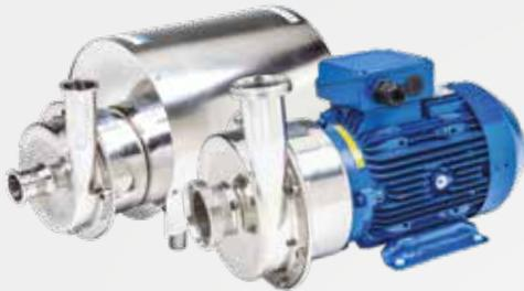
These pumps are open or semi open single stage centrifugal pumps, manufactured in high finish stainless steel AISI 316L. The range of applications is wide, from transfer of water to pumping of mild chemicals and low/medium viscous food products. To satisfy special needs, several options are available like flushed and/or lubricated seal, long coupled pump, draining system, heating jacket and hygienic shroud.
